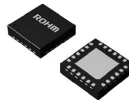
VQFN024V4040 4.00mm x 4.00mm x 1.00mm
