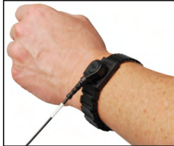
Wrist Strap Assembly. Cord snapped to Wristband
