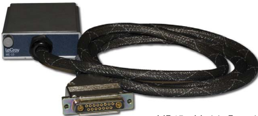
ME-15 – Module Extender Cable
