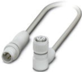
Sensor/Actuator cable, 4-position, PP-EPDM halogen-free, Gray RAL 7035, Plug straight M12, A-coded, on Socket angled M12, A-coded, Cable length: 0.3 m, Hygienic design, with plastic knurl
