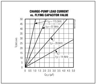
Figure 34. Load Current vs. CFLY Value for 2V<sub>DVDD</sub> - V<sub>AVDD</sub> ≥ 0.4V
