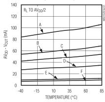
$\begin{array}{l} A:=R_{L}=5k\Omega,\,AV_{DD}=5V,\,DV_{DD}=3V & B:=R_{L}=5k\Omega,\,AV_{DD}=3V,\,DV_{DD}=2V\\ C:=R_{L}=10k\Omega,\,AV_{DD}=5V,\,DV_{DD}=3V & D:=R_{L}=10k\Omega,\,AV_{DD}=3V,\,DV_{DD}=2V\\ E:=R_{L}=100k\Omega,\,AV_{DD}=5V,\,DV_{DD}=3V & F:=R_{L}=100k\Omega,\,AV_{DD}=3V,\,DV_{DD}=2V \end{array}$
