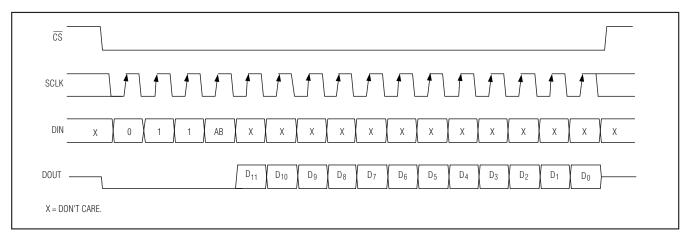
Figure 14. Read of DACA (AB = 0) or DACB (AB = 1) Input Register
