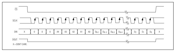
Figure 10. Variable Length Register-Mode Data-Write Operation
