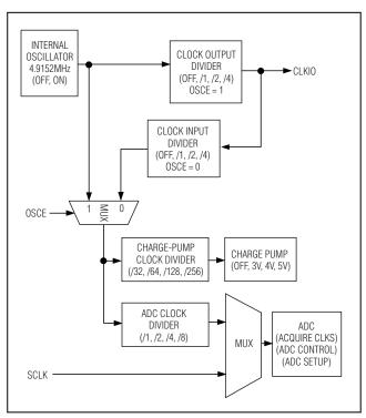
Figure 3. Clock-Divider Block Diagram
