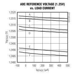
$\begin{array}{lll} A: T_A = -40^{\circ}C, \ AV_{DD} = 5V, \ DV_{DD} = 3V \\ B: T_A = -40^{\circ}C, \ AV_{DD} = 3V, \ DV_{DD} = 2V \\ C: T_A = +25^{\circ}C, \ AV_{DD} = 5V, \ DV_{DD} = 3V \\ C: T_A = +25^{\circ}C, \ AV_{DD} = 5V, \ DV_{DD} = 3V \\ F: T_A = +85^{\circ}C, \ AV_{DD} = 3V, \ DV_{DD} = 2V \\ \end{array}$
