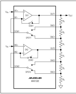
Figure 32. Programmable-Gain Instrumentation Amplifier, Switch Position 1
