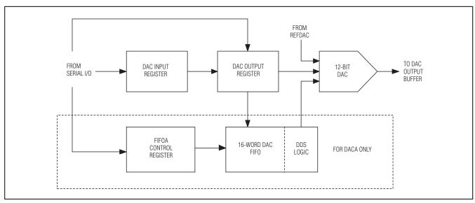
Figure 7. Detailed DAC and FIFO Block Diagram
