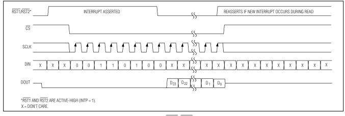
Figure 15. Read of Status Register to Clear Asserted Interrupt (RST1/RST2)
