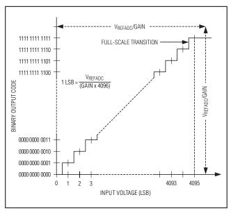
Figure 5. Unipolar Transfer Function
