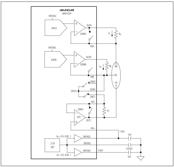
Figure 29. Three-Electrode Potentiostat Software-Switchable Single- or Dual-Channel Connection
