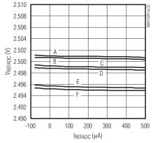
$\begin{array}{lll} A: T_A = -40^{\circ}C, \ AV_{DD} = 5V, \ DV_{DD} = 3V \\ B: T_A = -40^{\circ}C, \ AV_{DD} = 3V, \ DV_{DD} = 2V \\ C: T_A = +25^{\circ}C, \ AV_{DD} = 5V, \ DV_{DD} = 3V \\ C: T_A = +25^{\circ}C, \ AV_{DD} = 5V, \ DV_{DD} = 3V \\ F: T_A = +85^{\circ}C, \ AV_{DD} = 3V, \ DV_{DD} = 2V \\ \end{array}$
