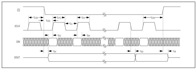
Figure 1. Detailed Serial-Interface Timing Diagram
