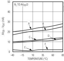
$\begin{array}{lll} A:=R_{L}=5k\Omega, AV_{DD}=5V, DV_{DD}=3V & B:=R_{L}=5k\Omega, AV_{DD}=3V, DV_{DD}=2V \\ C:=R_{L}=10k\Omega, AV_{DD}=5V, DV_{DD}=3V & D:=R_{L}=10k\Omega, AV_{DD}=3V, DV_{DD}=2V \\ E:=R_{L}=100k\Omega, AV_{DD}=5V, DV_{DD}=3V & F:=R_{L}=100k\Omega, AV_{DD}=3V, DV_{DD}=2V \end{array}$
