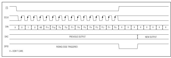
Figure 16. Write to DACA (AB = 0) or DACB (AB = 1) Input Register Followed by a DPIO DACA or DACB Load
