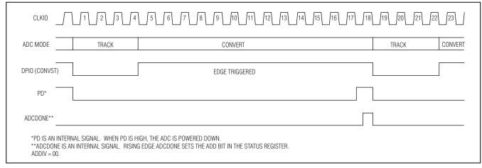
Figure 21. DPIO-Controlled ADC Conversion Start
