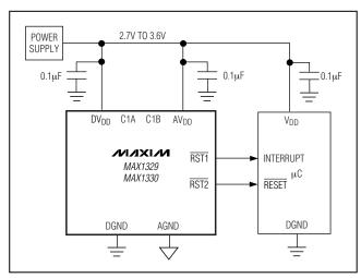
Figure 23. Power-Supply Circuit Using an External 3.0V Power Supply for DVDD and AVDD
