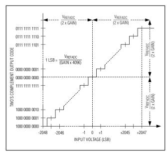
Figure 6. Bipolar Transfer Function
