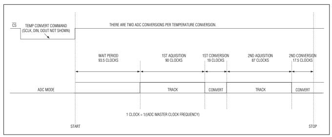
Figure 22. Temperature-Conversion Timing
