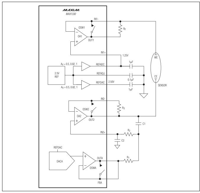
Figure 30. Two-Electrode Potentiostat with AC and DC Excitation
