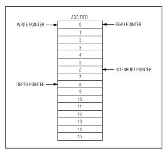
Figure 4. ADC FIFO
