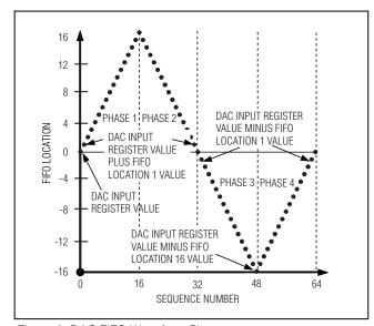
Figure 8. DAC FIFO Waveform Phases
