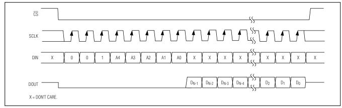
Figure 11. Variable Length Register-Mode Data-Read Operation
