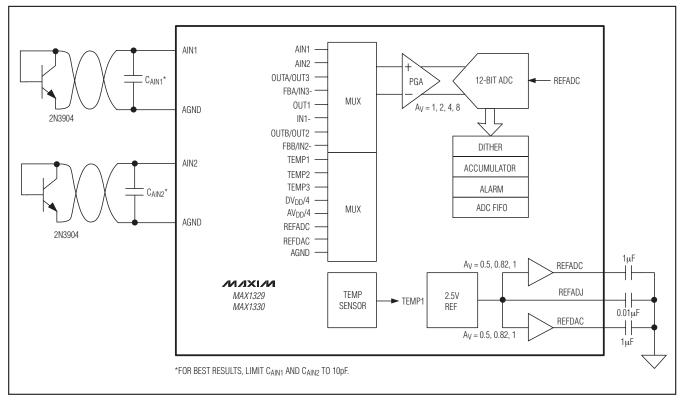
Figure 31. Temperature Measurement with Two Remote Sensors
