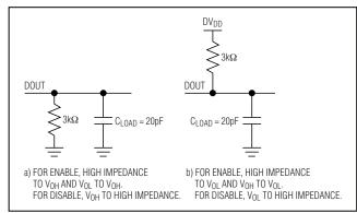
Figure 2. DOUT Enable and Disable Time Load Circuits
