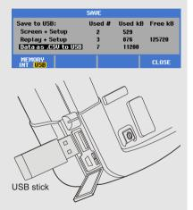
You can save data in .csv format to a USB stick. The saved .csv file can be used to analyze the data in e.g. FlukeView<sup>®</sup> ScopeMeter<sup>®</sup> or in Excel.
