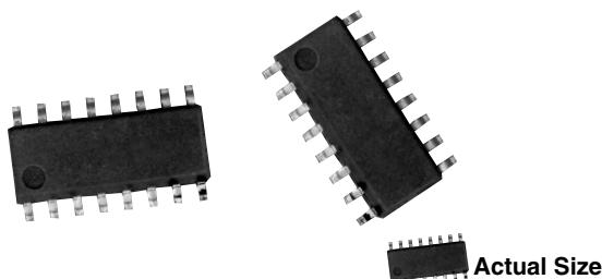
The NOMC series features a standard 14 pins and 16 pins narrow body (0.150") small outline surface mount style. It can accommodate resistor networks to your particular application requirements. The networks can be constructed with passivated nichrome (standard), or tantalum nitride <sup>(1)</sup> resistor films to optimize performance.
