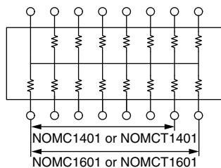
The 01 circuit provides a choice of 13 or 15 equal value resistors each connected between a common lead (14 or 16). Custom schematics available.
