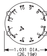
TERM. NOS. MOLDED ON HOUSING
