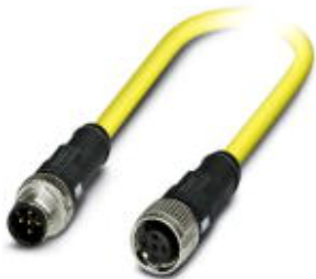
Sensor/Actuator cable, 5-position, PVC, Yellow RAL 1021, Plug straight M12-SPEEDCON, A-coded, on Socket straight M12-SPEEDCON, A-coded, Cable length: 0.5 m
