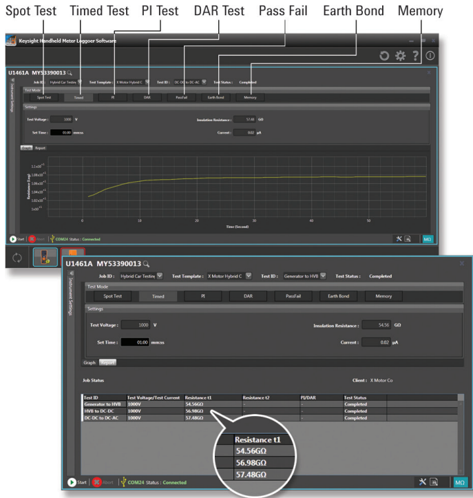
Figure 1. Keysight Handheld Logger Software Interface for Windows PC with guided operation and one button automatic report generation
