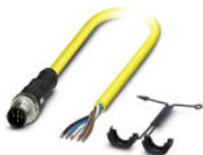
Sensor/Actuator cable, 5-position, PVC, yellow RAL 1021, Plug straight M12 SPEEDCON, A-coded, on free cable end, Cable length: 10 m
