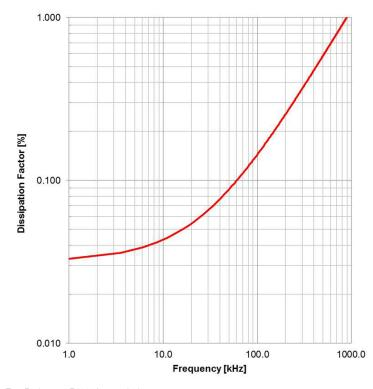
Test Equipment: E4991A or equivalent
