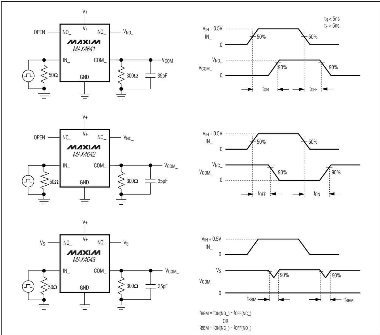
Figure 2. Switching Times
