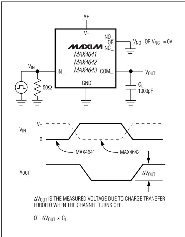
Figure 4. Charge Injection
