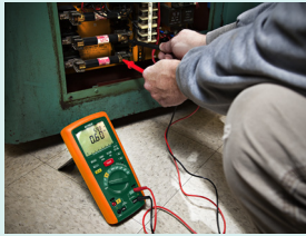
Checking voltage on a lathe
