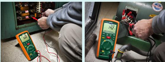
Checking voltage on a lathe
