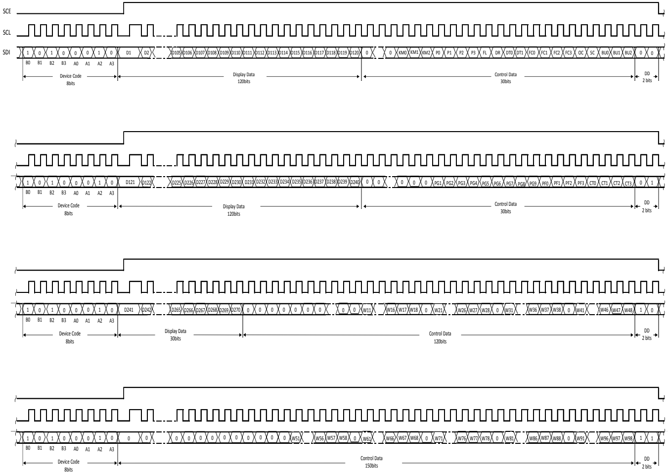
Figure 11. 3-SPI Data Transfer Format
