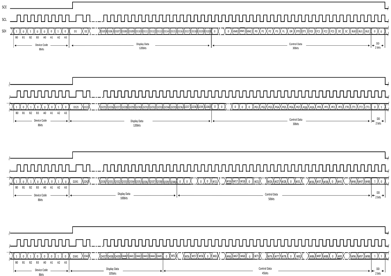
Figure 7. 3-SPI Data Transfer Format
